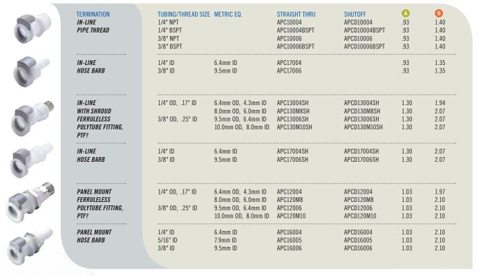
All measurements are in inches (millimeters) unless otherwise noted. Tubing must meet stated inside and outside diameters. tNOTE: CPC's Ferruleless Polytube Fitting terminations do not require ferrules to achieve a secure connection, which makes them easier to use and reuse. PTF fittings are designed for semi-rigid tubing, i.e., polyethylene, nylon, polyurethane, etc.
